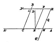
P, Q the points, draw QMQ', PLP' parallel to CB and CA, and make Q'M = QM and P'L = PL.
